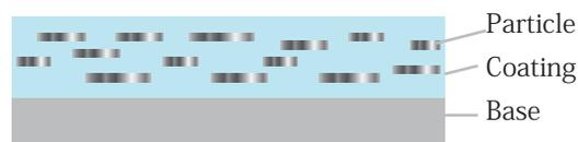
○High flow rate, single layer: Poor alignment, low brightness and flop.
