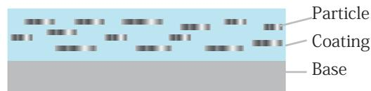
○Thin coating: good alignment, high brightness and high flop.
