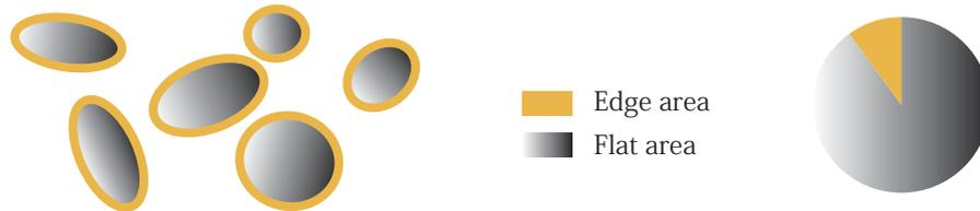
○Irregular particle: Jagged edges produce more diffused reflection and less brightness.
